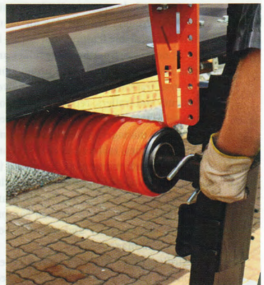
2 Installation is straightforward and service can be performed by a single person using a socket wrench
